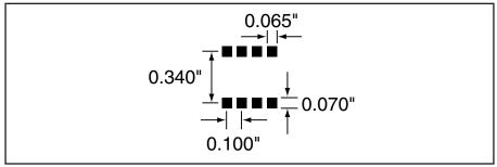
Figure 9: Recommended PCB Layout
