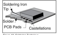
Figure 10: Soldering Technique
