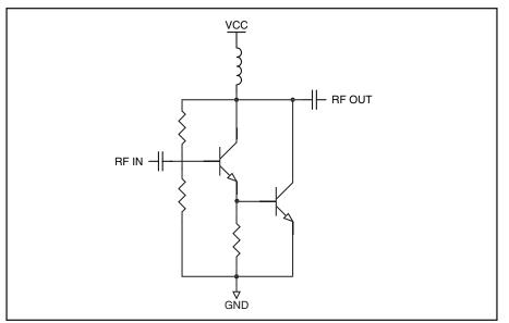
Figure 4: BBA Series Amplifier Schematic
